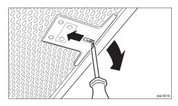
If the filter is incorrectly installed, insert a small screwdriver into the slit along its edge to disengage it from the casing.
